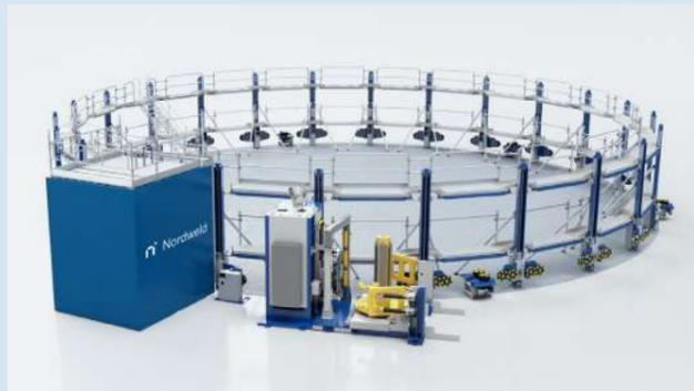
1. Place the annular and bottom plates at the foundation. Place the equipment on the annular plates and assemble the Lift Jacks including Wheel Trolleys. Place the vertical bending machine / decoiler / plate track in position.
