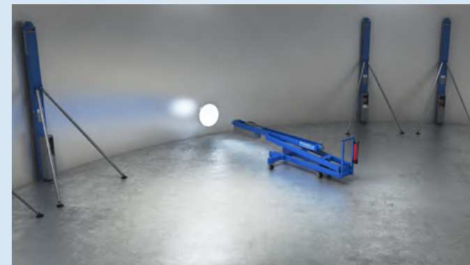
9. Remove the equipment and place the tank at the bottom and dismantle the Lift Jacks.
