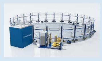
1. Place the annular and bottom plates at the foundation. Place the equipment on the annular plates and assemble the Lift Jacks including Wheel Trolleys. Place the vertical bending machine / decoiler / plate track in position.
